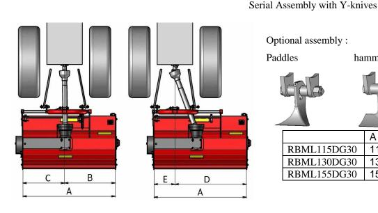
Optional assembly : Paddles scarificators hammers В С D Е Α RBML115DG30 115 55 60 85 30 RBML130DG30 130 60 100 30 70 78 RBML155DG30 155 77 107 48
